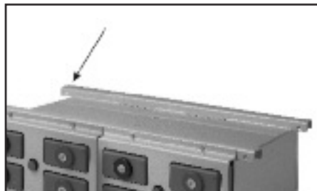
Figure 4: Recommended Frame Ground Location
