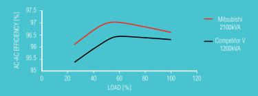
The 9900CX Series is optimized around typical loads of 25% to 75% while delivering high efficiencies across all hyper-scale load levels.
