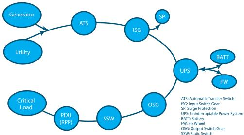
SSW: Static Switch PDU: Power Distribution Unit Critical Load: Anything Needing Power Protection
